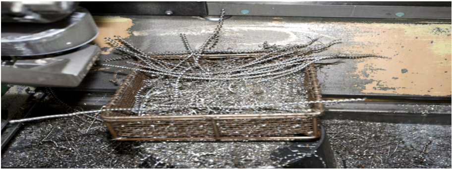
Figure 1.7: showing long shiny Swarfs in a Tray in the machining centre compartment.
